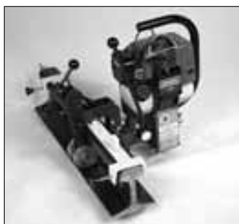
Distance gauge and rail drilling machine mounted on rail
