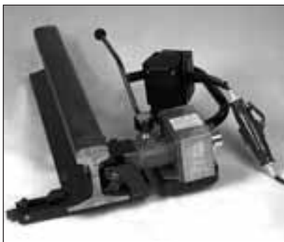
SBM-E 230 V with rail fastening device BSF1
